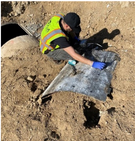
West Yost performed ultrasonic testing of steel pipe sample as part of condition assessment.
