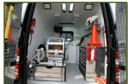
Photograph 2-1 EnviroSight CCTV Inspection and Pipeline Scanning Truck
