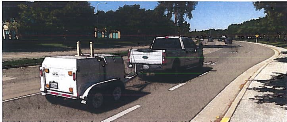
Photo 1: GMU's falling-weight deflectometer in action on a City of Irvine pavement evaluation project (2022).
