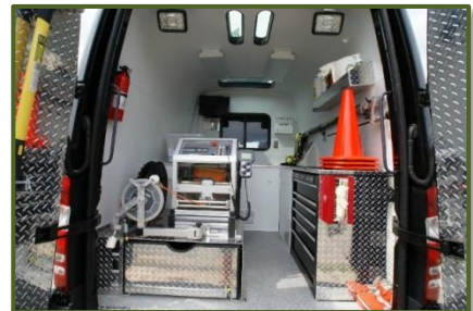
Photograph 2-1 Envirosight CCTV Inspection and Pipeline Scanning Truck
