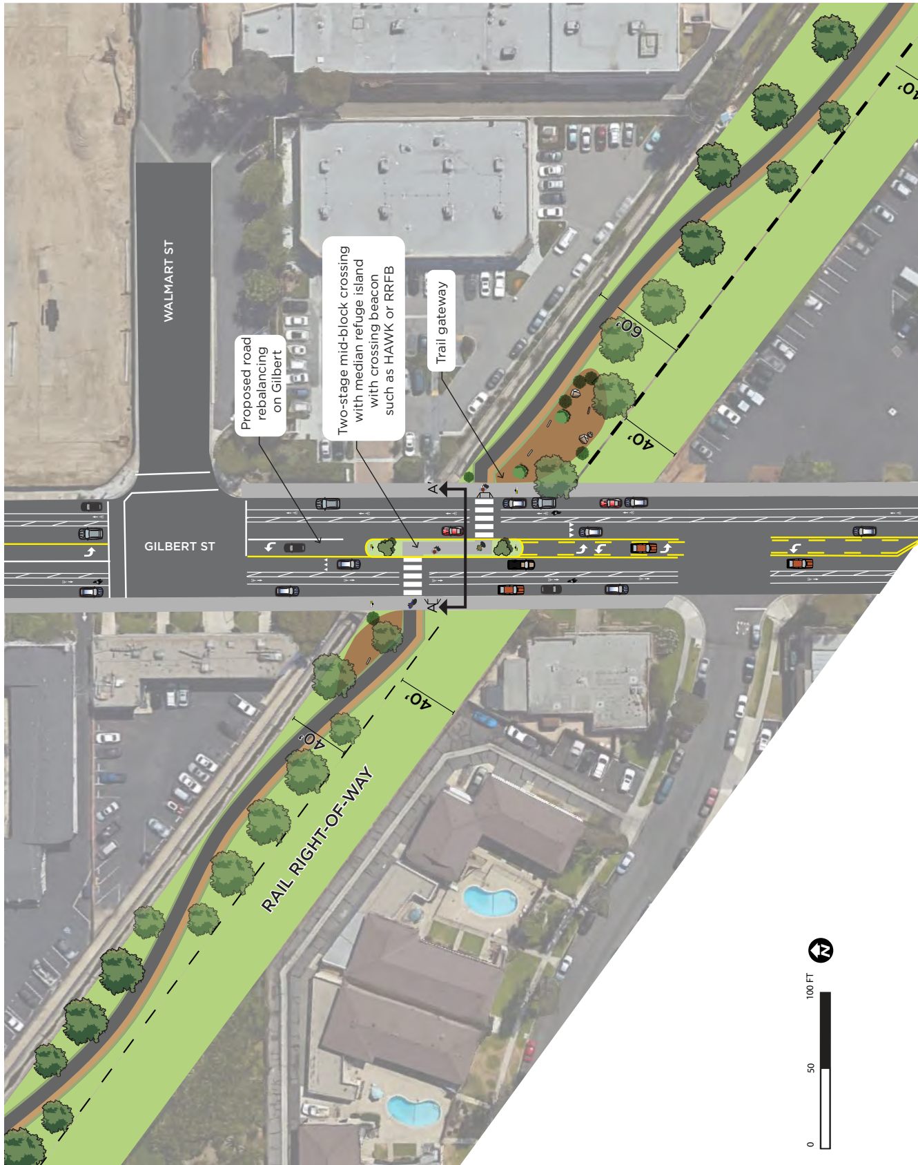
Figure 8-5: Proposed Concept of PE ROW Trail alignment and crossing at Gilbert Street.
