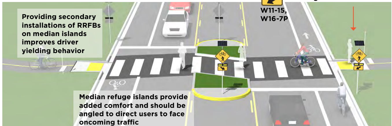
Figure 5-4: Best Practice Design Guide for Median Refuge Islands
