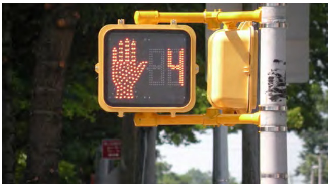
Pedestrian countdown signals provide timing information to pedestrians crossing the street and communicate pedestrian right of way to drivers
