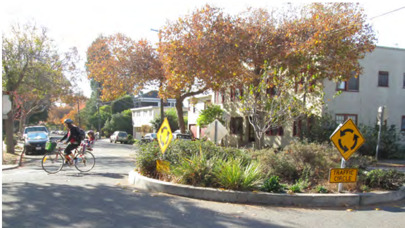
Right: Long Beach's custom signage. A neighborhood greenway, traffic circle, and signage in Long Beach, CA. Yield signs and traffic circles caution drivers to slow down, pedestrian crossing signage creates a safer walking environment, and bicycle signage and pavement markings make a safer and more convenient bicycle environment
